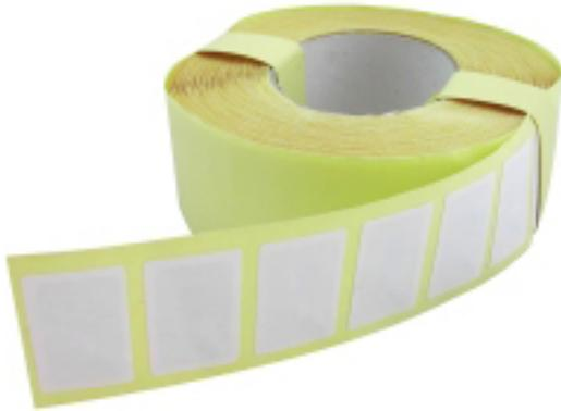
The MIFARE Ultralight chip from NXP, in sticky label format. Operates at 13.56 MHz wireless frequency, according to the ISO 14443A standard. Contains 48 bytes of usable read/write memory, with no security protection.
